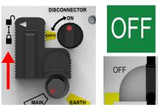
3 : Rotate the 'DISCONNECTOR' anticlockwise to 'EARTH'.
