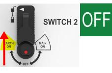
3: With the operating handle on the switch boss, rotate clockwise until the switch closes 'EARTH-ON'
