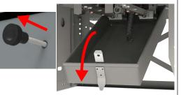
**4** : Insert the operating handle into the star point earth bar and pull down away from the bushings.
