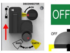
5: Rotate the DISCONNECTOR clockwise to 'ON' Switch.
