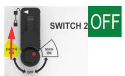
3: With the operating handle on the 'SWITCH 2' boss, rotate clockwise until the switch closes 'EARTH ON'.
