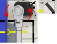
**3.** Rotate the Disconnector selector knob anticlockwise to '**EARTH**'. With the operating handle on the Disconnector boss, rotate anti-clockwise to approximately 60° from '**OFF**' to '**EARTH**'.
