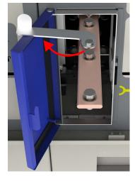
NOTE: The relevant function cannot be removed from 'EARTH-ON' until the test access door is closed.
