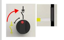
**2.** With the operating handle on the switch boss, rotate anti-clockwise 90° until the load switch closes to 'OFF'.
