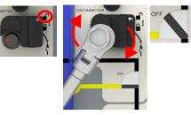
3. Rotate the Disconnector Selector knob Clockwise. Insert operating handle on to the 'Disconnector' boss and rotate clockwise approximately 60° from 'OFF' to 'ON'.
