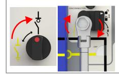
4. With the operating handle on the circuit breaker boss, rotate the ratchet mechanism one full revolution clockwise. At the end of the revolution the circuit breaker will close to 'ON'.
