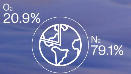
Obtainable globally, synthetic air is 79.1% nitrogen and 20.9% oxygen, with a purity of 5.0 (99.9990% pure).
