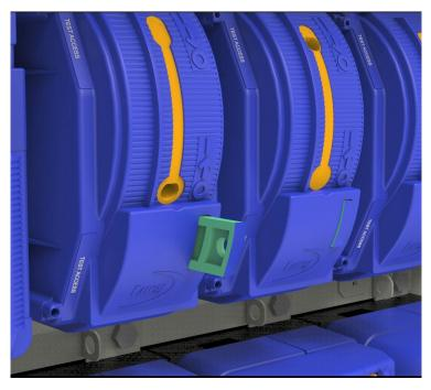
4. To close the disconnector links, return the handle to the top position. With the palm of the hand, exert upward pressure on the underside of the black handle. Disconnector will "fire" and a loud "clunk" will be heard
