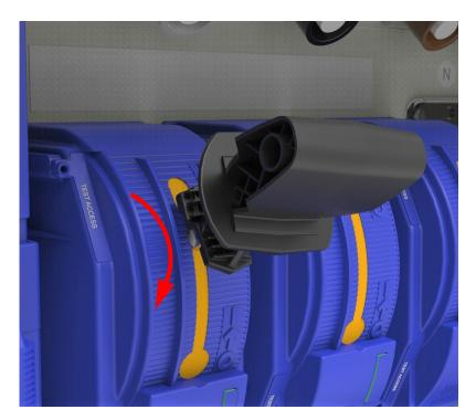
3. Disconnector is now at fully open/off position as witnessed by the extended green tab. Note the provision of a hole in each of the disconnector shuttle tabs for the padlockable lock off bar.
