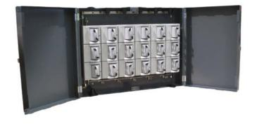
Wall mounting cabinets which accept single incoming supply and provide up to 5 outgoing J type triple pole fuse ways for indoor applications only.
