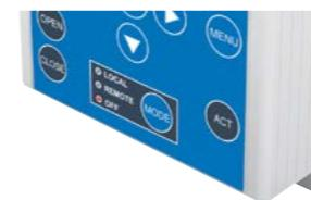
Three operation modes are available; control capability off, local and remote. The status of these operating modes is indicated by LEDs, and can be communicated to the SCADA. These operating modes can be switched using the Gemini 3 HMI option. Binary inputs can also be configured to provide off / local/ remote as an alternative to the HMI.
