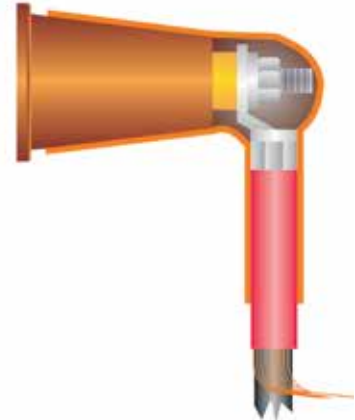
Heat shrink insulating bushing boot
